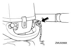
After stopping the engine, tighten the air vent screw on the fuel tank cap and set the fuel cock lever or knob to the closed position, if equipped.
